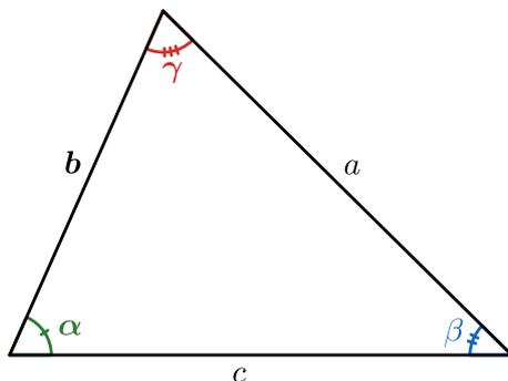
$$\alpha + \beta + \gamma = 180^\circ \implies \beta = 180^\circ - \alpha - \gamma$$
