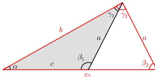
$$\begin{aligned} \beta_1 &= \pi - \beta_2; \quad \beta_1 \in \text{II} & \beta_2 &= \arcsen\left(\frac{b}{a} \sen \alpha\right); \quad \beta_2 \in \text{I} \\ \gamma_1 &= 180^\circ - \alpha - \beta_1 & \gamma_2 &= 180^\circ - \alpha - \beta_2 \\ c_1 &= \sqrt{a^2 + b^2 - 2ab \cos \gamma_1} & c_2 &= \sqrt{a^2 + b^2 - 2ab \cos \gamma_2} \end{aligned}$$
