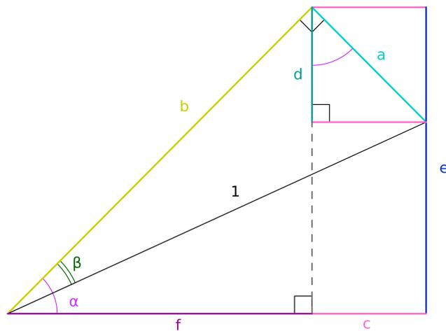
$$\begin{aligned} \operatorname{sen} \beta &= a \\ \operatorname{cos} \beta &= b \\ \operatorname{sen} \alpha &= \frac{e}{b} = \frac{c}{a} \\ \operatorname{cos} \alpha &= \frac{f}{b} = \frac{d}{a} \end{aligned}$$
