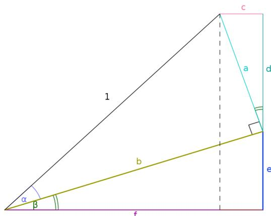
$$\begin{aligned}\operatorname{sen} \alpha &= a \\ \operatorname{cos} \alpha &= b \\ \operatorname{sen} \beta &= \frac{e}{b} = \frac{c}{a} \\ \operatorname{cos} \beta &= \frac{f}{b} = \frac{d}{a}\end{aligned}$$
