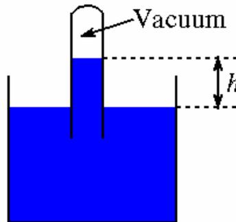
$$\text{water } (\rho = 1000 \text{ kg/m}^3) : h = \frac{P_{\alpha}}{\rho g} = \frac{1.013 \times 10^5 \text{ Pa}}{10^3 \text{ kg/m}^3 \cdot 9.8 \text{ m/s}^2} = 10.3 \text{ m}$$
